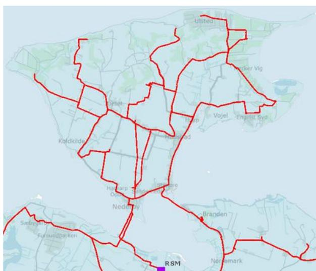
Figure 7: Electricity cables on Fur and the station in Risum (RSM) (Source: N1)
